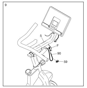
10. Connect the console wire (E) to the Upper Wire (90). IMPORTANT: The wire connectors should slide together easily and snap into place with an audible click. If they do not, turn one connector and try again. Then, insert the connectors into the Console Mount.
