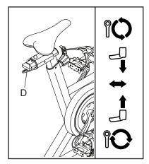
Note: The adjustment handle (D) functions like a ratchet. Turn the adjustment handle in the desired direction, pull it downward, turn it in the opposite direction, push it upward, and then turn it in the desired direction again. Repeat this process as many times as necessary.
