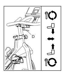
Note: The adjustment handle (D) functions like a ratchet. Turn the adjustment handle in the desired direction, pull it downward, turn it in the opposite direction, push it upward, and then turn it in the desired direction again. Repeat this process as many times as necessary.
