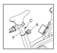
into one of the adjustment holes (C) in the seat post, and tighten the adjustment knob. Move the seat post upward or downward slightly to make sure that the adjustment knob is engaged in an adjustment hole.
