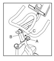
dlebar post, and tighten the adjustment knob. Move the handlebar post upward or downward slightly to make sure that the adjustment knob is engaged in an adjustment hole.
