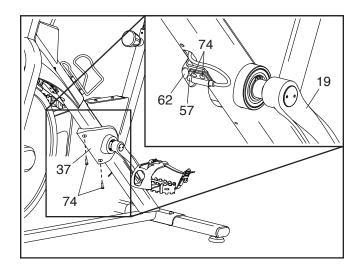
Next, locate the Reed Switch (57). Slightly loosen the two indicated M4 x 12mm Blunt Screws (74). Then, turn the Left Crank Arm (19) until a Magnet (62) is aligned with the Reed Switch. Slide the Reed Switch slightly toward or away from the Magnet. Then, retighten the Blunt Screws.
