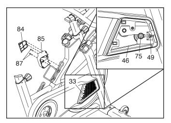
Next, loosen, but do not remove, the M10 Flange Nut (75) on each side of the exercise bike (only one side is shown).
