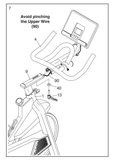
8. Tighten an ST4 x 15mm Blunt Screw (94) into the underside of the Handlebar Post (9).
