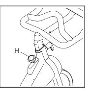
IMPORTANT: When the exercise bike is not in use, tighten the brake knob (H) completely.
