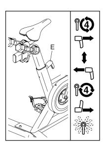
Make sure that the adjustment handle is engaged in an adjustment hole. Then, pull the adjustment handle outward, turn it so that it points downward as shown, and then release it.
