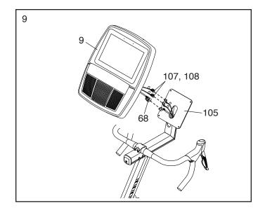
10. **Tip: Avoid pinching the wires.** Attach the Console (9) to the Handlebar Carriage (105) with four M4 x 12mm Screws (111); **start all the Screws, and then tighten them.**
