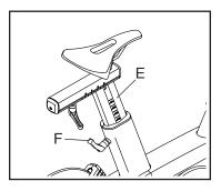
post (E), loosen the adjustment handle (F), move the saddle post upward or downward, and then retighten the adjustment handle. When you are finished tightening the adjustment handle, make sure that the end of the adjustment handle is pointing upward.
