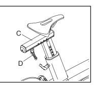
Note: The adjustment handle (D) functions like a ratchet. Turn the adjustment handle in the desired direction, pull it outward, turn it in the opposite direction, push it inward, and then turn it in the desired direction again. Repeat this process as many times as necessary.
