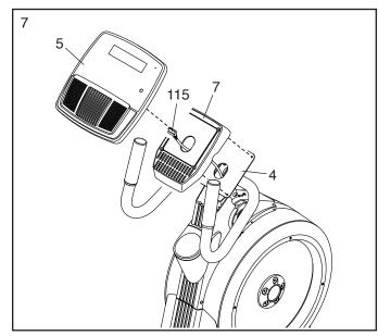
8. Avoid pinching the wire. Attach the Console (5) and the Console Cover (7) to the Console Bracket (4) with four M4 x 22mm Screws (107). Start the two upper Screws first, and then start the two lower Screws; then, tighten all four Screws.
