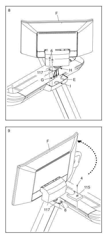
10. Rotate the console assembly (F) back to its original position. Firmly tighten the two M6 x 25mm Screws (6) that you attached in step 8.
