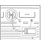
up to a few minutes for the console to be ready for use. IMPORTANT: In an emergency, the key can be pulled from the console, causing the walking belt to slow to a stop. Test the clip by carefully taking a few steps backward; if the key is not pulled from the console, adjust the position of the clip.
