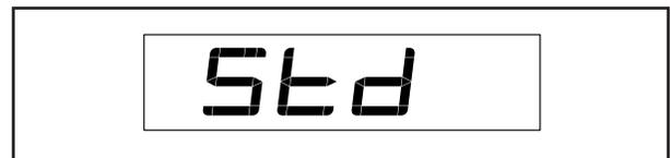
**Display Test**—This screen is intended to be used by service technicians to identify whether the display is working correctly.
