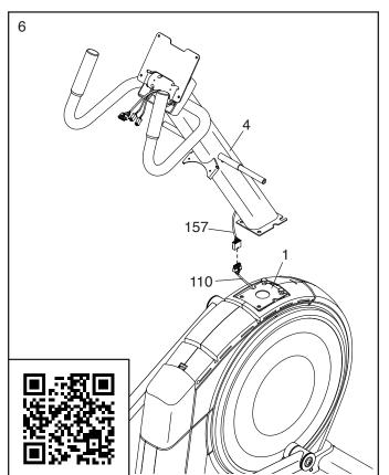
7. **Avoid pinching the wires.** Have a second person hold the Upright (4) on the Frame (1).
