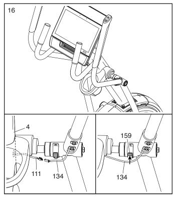
17. **Avoid pinching the wires.** Orient a Lower Tray Cover (81) as shown, and hold it near the Right Control Wire (134). Attach the Lower Tray Cover to the right side of the Accessory Tray (37) with two M4 x 16mm Screws (101).
