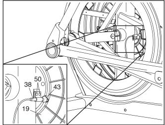
Next, slightly loosen the indicated two M4 x 12mm Self-tapping Screws (50). Slide the Reed Switch (38) slightly closer to or away from the Magnet (43), and then retighten the Self-tapping Screws.
