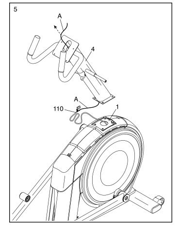
6. **Tip: Avoid pinching the Upper Wire (110).** Have a second person hold the Upright (4) on the Frame (1).
