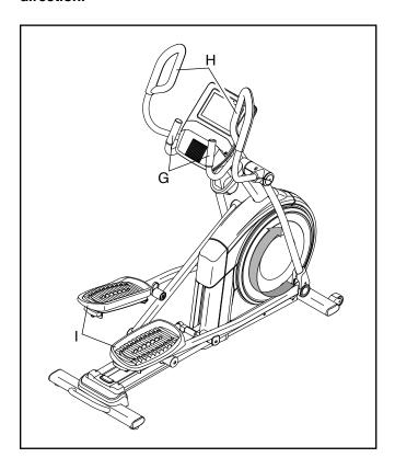
To dismount the elliptical, wait until the pedals (I) come to a complete stop. **Note:** The elliptical does not have a free wheel; the pedals will continue to move until the flywheel stops. When the pedals are stationary, step off the higher pedal first. Then, step off the lower pedal.
