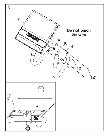
Identify the Console Lower Cover (120), and press it onto the back of the Console (5). Then, press the Console Upper Cover (119) onto the back of the Console. Do not pinch the console wire (A).
