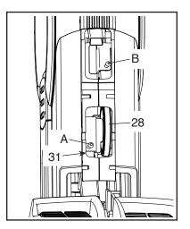
Adjustment Screw (B). Tighten the upper Adjustment Screw two turns; this will tighten the Small Drive Belt (28).
