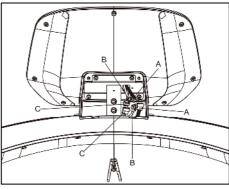
9. Use 2 x M8\*16 (182) screws with flat washers (183) to fasten the console screen assembly to the console base.
