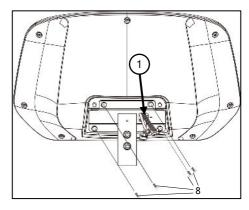
8. Place the console screen assembly on the console base. Connect the console connections A to A, B to B and C to C, respectively.
