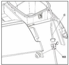
6. Use 6 x M10\*16 (187) screws with a flat washer (189) to fasten the uprights to the Console. Lightly fasten all screws until all screws have been aligned. Then tighten all screws in step 4 and 6.
