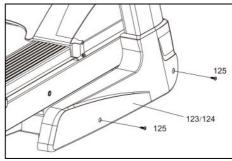
12. Remove the lock plate securing the base frame in the down position.
