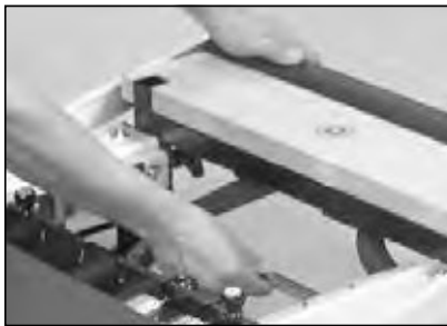
1. Move the chrome adjuster bar [8] to set the footbar [7] into the lowest position.
