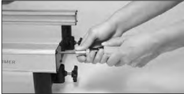
2. Using a Phillips screwdriver, remove stopper plates.
