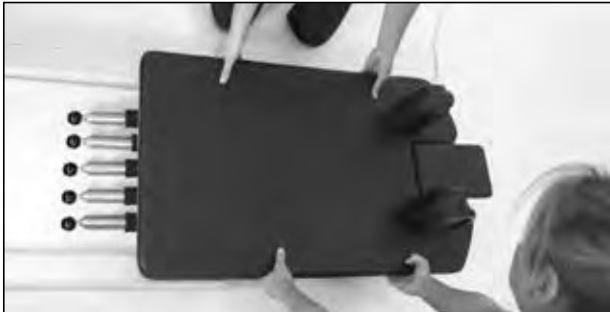
3. Detach all springs from gearbar. Carefully slide carriage out of aluminum rails keeping carriage level until completely free of rails. Turn carriage over, ensuring rollers are secure and do not come in contact with the floor.
