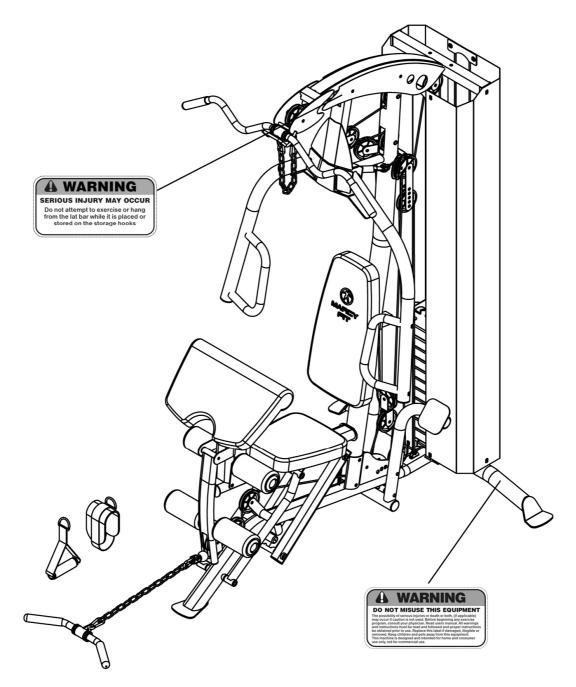
The warning labels shown here have been placed on the Rear Base and Upper Frame. If the labels are missing or illegible, please contact customer service by email: service.international@tunturi-fitness.com for replacements. Apply the labels in the location shown.
