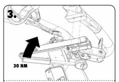
MOUNT THE HANDLEBAR TO THE STEM WITH 2 COUNTER SUNK HEX BOLTS. TIGHTEN TO 30 NM WITH A TORQUE WRENCH. THE BOLTS ARE PRE-COATED WITH A THREAD LOCK WHEN TIGHTENED FOR THE FIRST TIME. IF THE BOLTS SHOULD LOOSEN, GLUE BOLTS WITH LOCKTITE (R) 2701 UPON RETIGHTENING.
