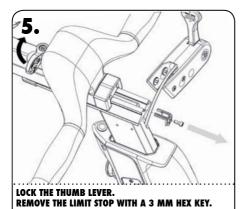
NEVER PULL THE HANDLEBAR TOWARD THE SEAT WHEN THE LIMIT STOP IS REMOVED. THIS WILL
