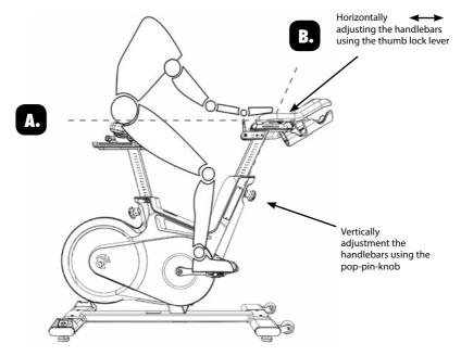
The next step is to adjust the horizontal position of the handlebars as precisely as possible to your height. An ideal and comfortable seating position for inexperienced riders is achieved if your back assumes an inclination angle of 45° in reference to the horizontal line (A).
