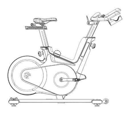
During the assembly process, the warning label on the bike must be replaced by a warning label in the native language of the country in which the indoor cycle is being used.
