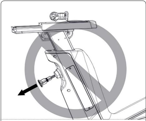
THE VERTICAL HANDLEBAR STEM OF THE INDOOR CYCLE IS SPRING LOADED AND WILL EXTEND QUICKLY UNLESS THE HANDLEBAR IS MOUNTED ONTO THE STEM. EXTENSION OF THE STEM WITHOUT THE MOUNTED HANDLEBAR MAY CAUSE INJURY OR/AND DAMAGE TO THE INDOOR CYCLE.
