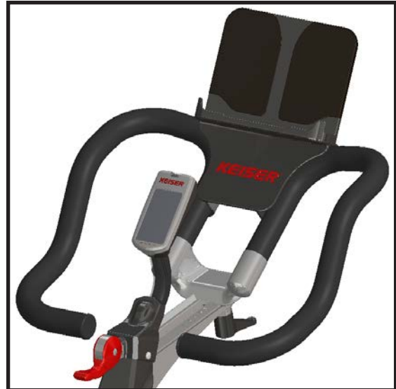
Figure 20. The assembled handlebar and device holder
