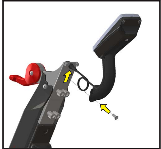
Figure 12. Attach the Computer to the Handlebar Tube
