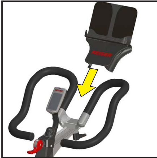
Figure 19. Assemble the device holder to the handlebar
