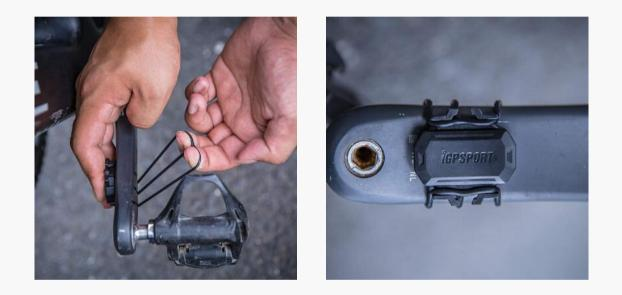
C) Finally, connect HOLOFIT to the cadence sensor using Bluetooth. It will automatically be visible in the pairing settings on HOLOFIT.
