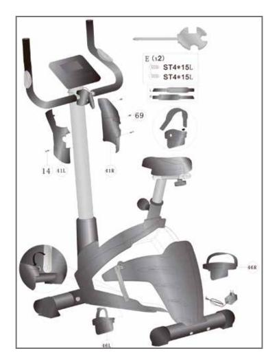
(2) Attach the pedals (46L) and (46R) to the pedal cranks.
