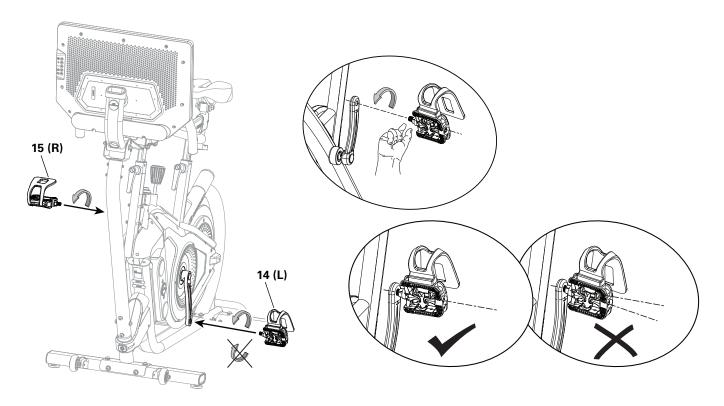
With the Pedal started by several hand turns into the Crank Arm, fully tighten it with the 15 mm Wrench.
