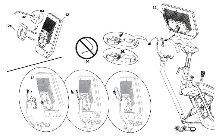
**NOTICE:** Push the extra wire down into the Console Mast. Reinstall the console hardware (\*). Install the Console Mast End Cap (13) and Console mast cover (12a). Do not pinch or cut the cables.
