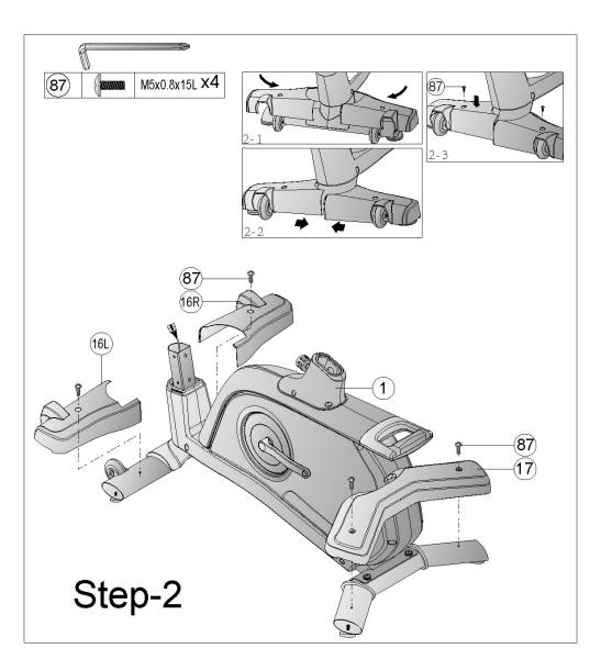
1) Assemble the front stabilizer cover (16L&16R) and rear stabilizer cover (17) onto the front and rear stabilizer by Bolt (87) as fig 2-1,2-2 and 2-3.
