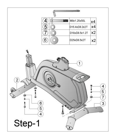
1) Assemble the front stabilizer (2) and the rear stabilizer (3) to the main frame (1) by Allen bolt (4), Spring washer (5), Flat washer (6) and Flat washer (7).
